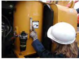
Check for proper hydraulic fluid level.
