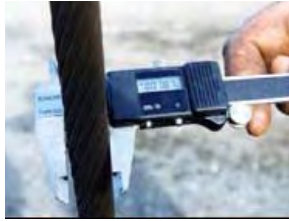
MEASURE WIRE ROPE TO CHECK FOR WEAR
