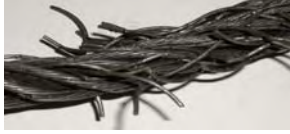
Heavy loads over small sheaves
